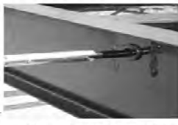
Fig. 2-Through Frame Crank Extension w/Pin
