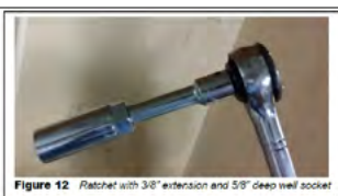
Figure 12 Ratchet with 3/8" extension and 5/8" deep well socket
