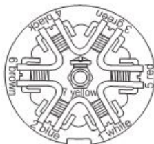
7-way trailer plug - Car end, rear view
