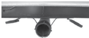
Black/Grey tank drain & valves
